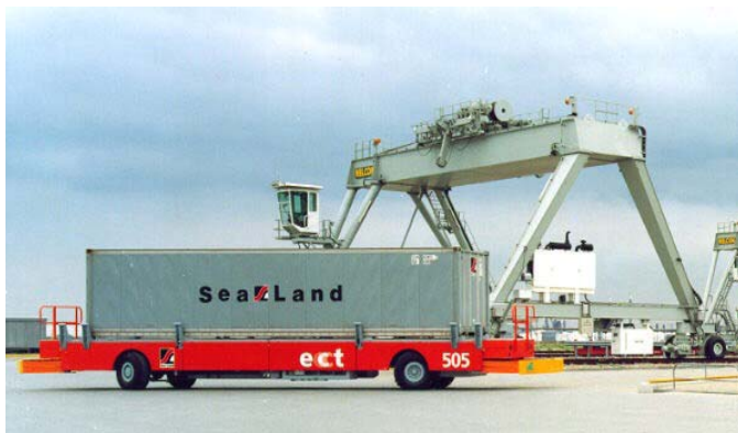
Figure 6. AGV operating in European Combined Terminal (ECT) in Rotterdam, Netherlands (obtained from Frog Systems website)
