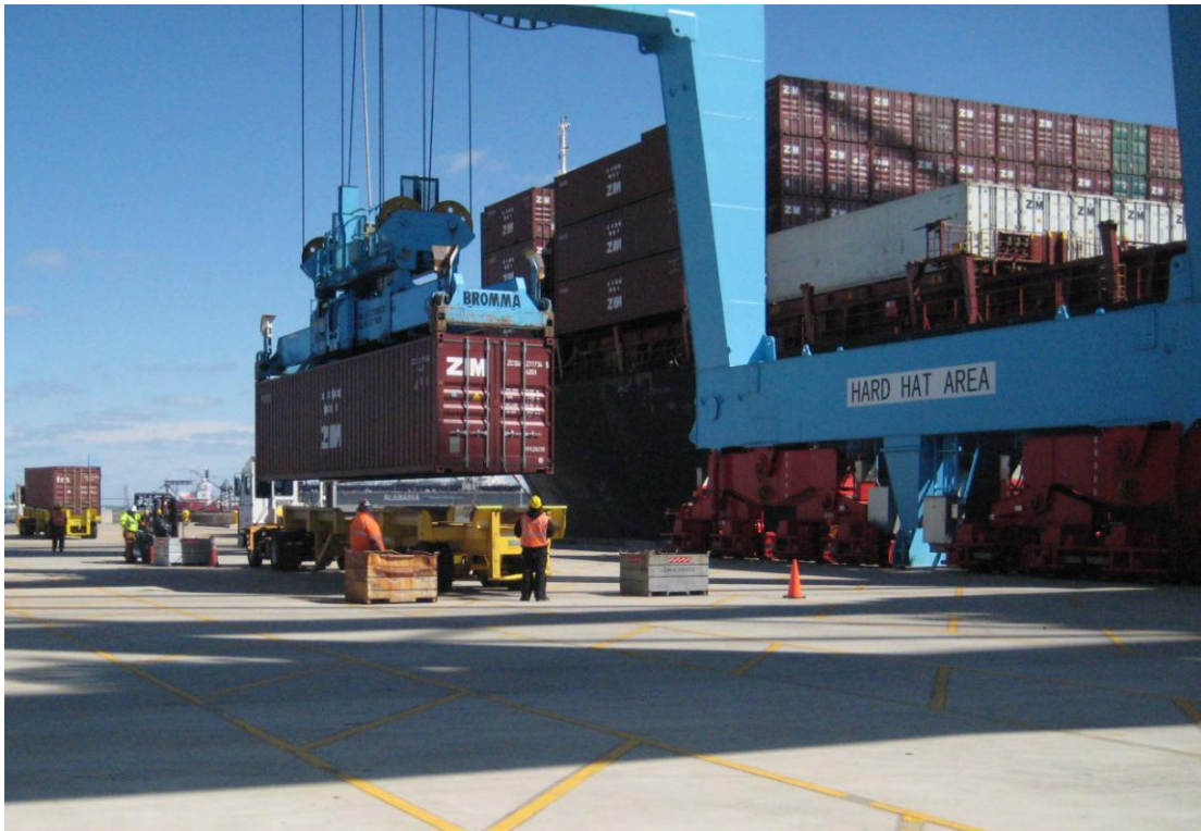
Figure 2. One of two ship cranes unloading container onto a cart
